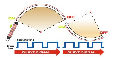
The FluiLub wheel flange lubrication system is designed as single line system. This means: Less wear, little maintenance requirements and therefore low life-cycle costs.
