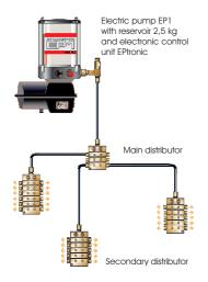
The electronic control of the central lubrication is adapted to the operating conditions of the vehicle and activates the pump in defined intervals.
